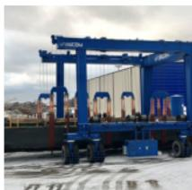
Suomenlahden Telakka Oy focuses its activities on the maintenance, repair and conversions of coastal tonnage ships. The yard is located in Port of Valko, Loviisa. Using a boat hoist – the biggest in the Nordics so far – allows the repaired vessel to be lifted conveniently out of water and docking or launching in less than 1h. The yard's warm, well illuminated and efficient travers crane outfitted hall provides high-class quality and productivity for the customers.
